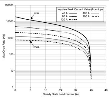
Figure 3. Maximum Cycle Rate for Multiple Paths Closed
